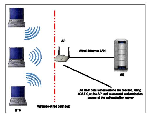
Figure 3-3. IEEE 802.1X Port-Based Access Control
