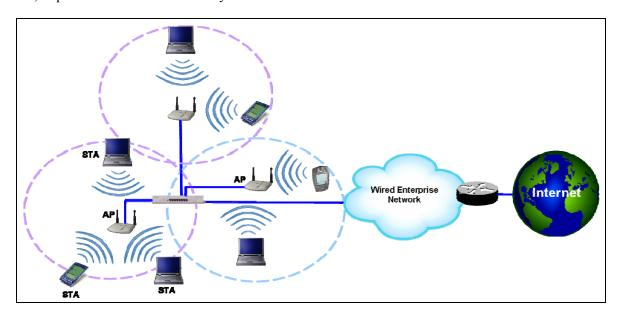
Figure 2-3. Extended Service Set in an Enterprise
