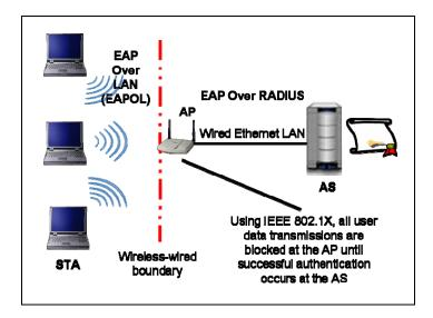
Figure 6-2. Illustration of EAP-TTLS Environment
