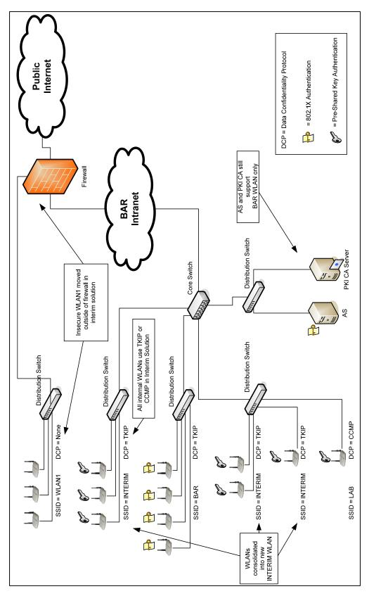
Figure 9-3. BAR WLAN Interim Solution
