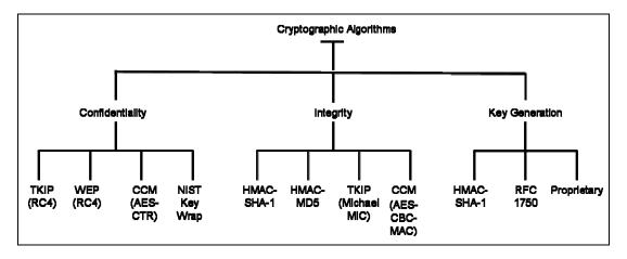
Figure 4-3. Cryptographic Algorithms Used in IEEE 802.11<sup>26</sup>
