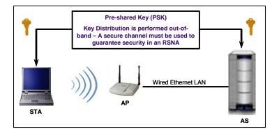
Figure 4-5. Out-of-Band Key Distribution for the PSK
