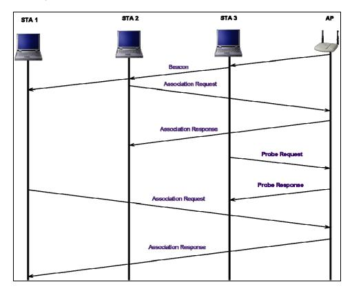
Figure 5-2. Multi-STA WLAN Flow Diagram
