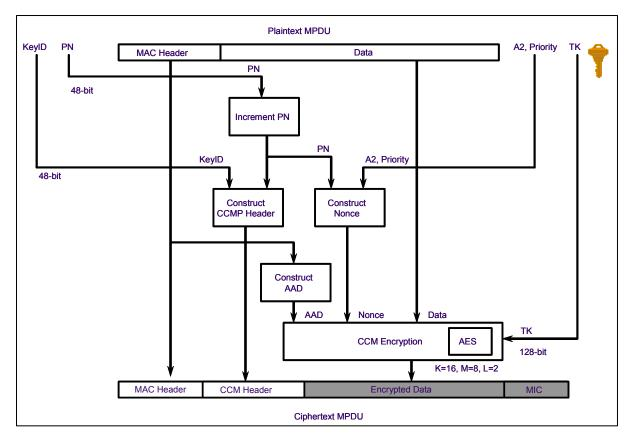
Figure 4-7. CCMP Encapsulation Block Diagram
