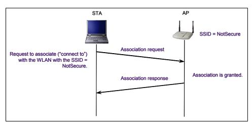
Figure 5-1. Typical Two-Frame IEEE 802.11 Communication
