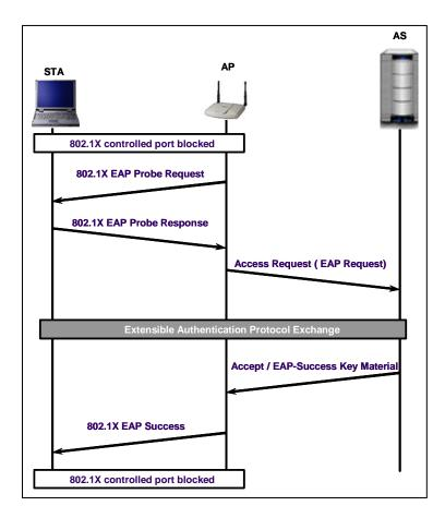
Figure 5-10. Authentication Phase of Operation
