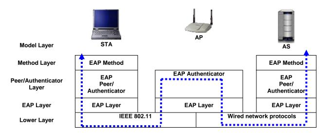
Figure 6-5. EAP Traffic Flow in IEEE 802.11 RSN
