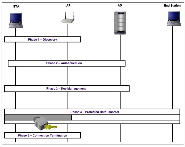
Figure 5-4. Five Phases of Operation
