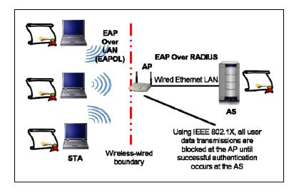
Figure 6-1. Illustration of EAP-TLS Environment
