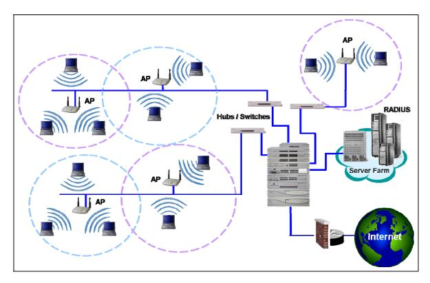
Figure 5-13. Typical Enterprise with Multiple APs, STAs, and an AS
